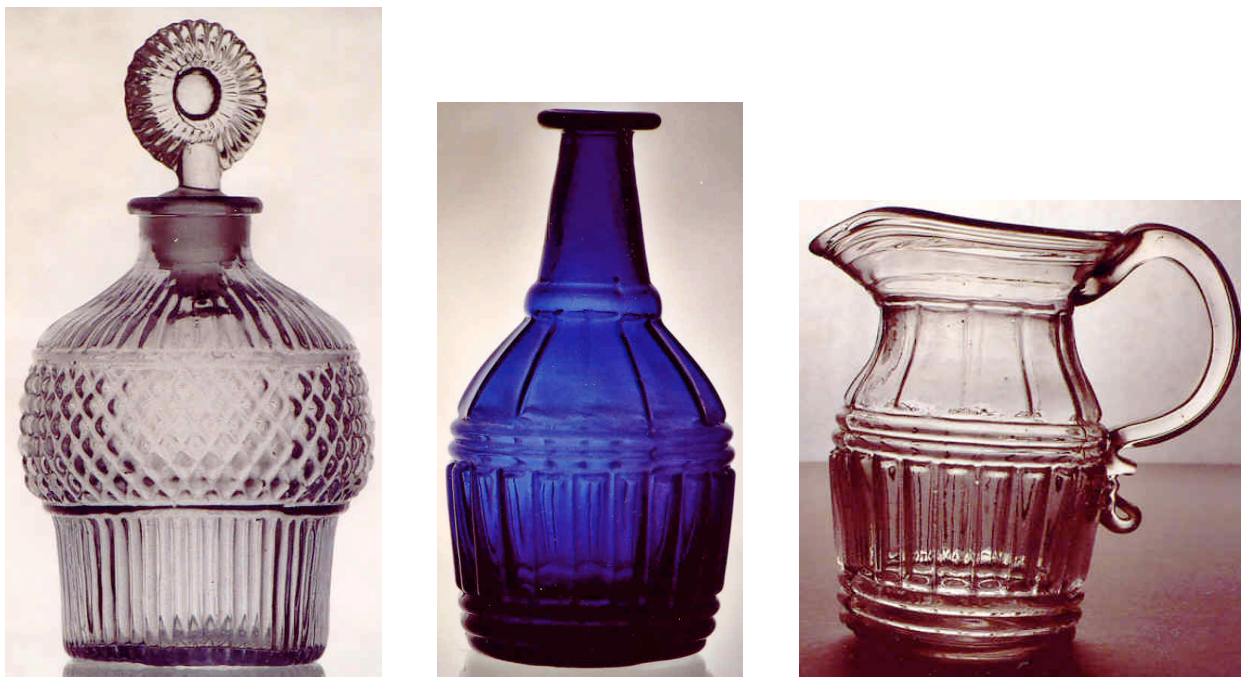
Figure 1. Three pieces of blown three mold glass: (a) a clear GII-18 bottle; (b) and (c) two pieces from the same GI-29 mold. While (b) obtained its final shape in the mold, the neck of (c) was widened and shaped to form the body of a pitcher, and a rod of glass was added to form a handle.
