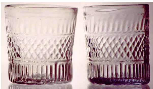
Figure 3: Siblings but not twins. Two small tumblers, blown in the same mold, but with slight differences in their shapes. This mold was used in Keene, New Hampshire, primarily to make inkwells.
